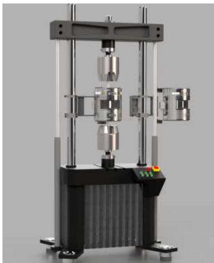
Twin furnaces column mounted (servohydraulic/servolectric)
