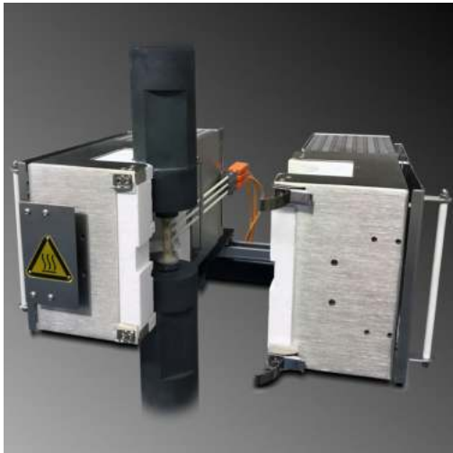
Three zone Silicon Carbide heated 'short furnace' SF2151A with rear mounted specimen thermocouple assembly. Designed for a maximum element temperature of 1400°C
