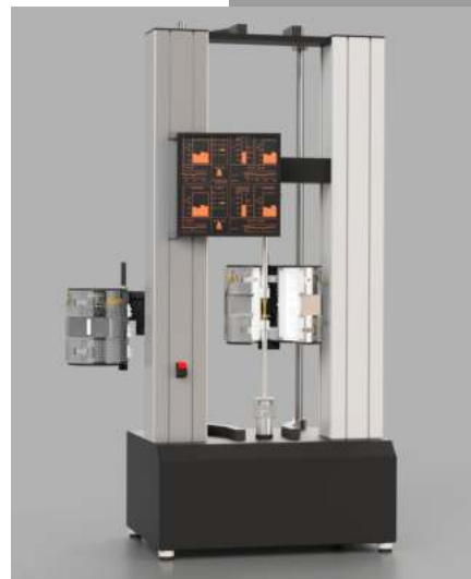
Twin furnaces attached to rear mounted pillars (electromechanical)
