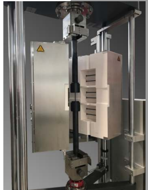
Three zone Molybdenum Disilicide heated split furnace MDS2296A. Designed for a maximum furnace temperature of 1550°C
