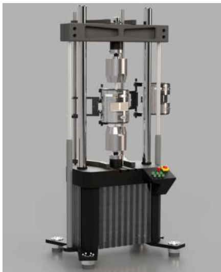
Twin furnaces attached to rear mounted pillars (servohydraulic/servolectric)
