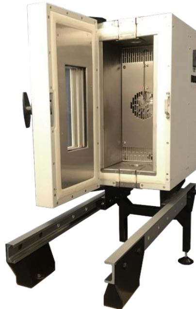
Trolley type roller mounting system, allowing the chamber to be moved clear of the test space and to be used across multiple test frames having the same test space height in relation to floor level
