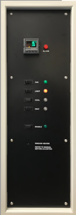
Rear side panel mounted control interface of the type utilised on larger 'floor model' environmental chambers
