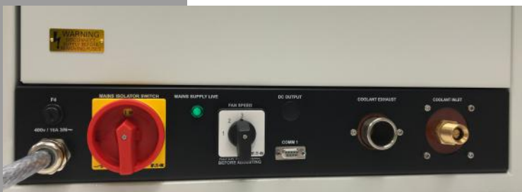
Rear of floor model environmental chamber showing mains isolator, liquid Nitrogen inlet/exhaust, fan speed selector and communications interface
