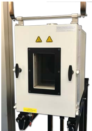
Compact -150°C - 600°C chamber with spring supported fully removable door, for use with close proximity DIC system
